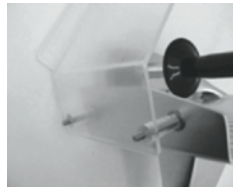
2. Attach the hand guard.
